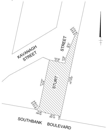
THE ROAD PROPOSED TO BE DISCONTINUED IS SHOWN HATCHED AND IS ENCLOSED BY THICK CONTINUOUS LINES
